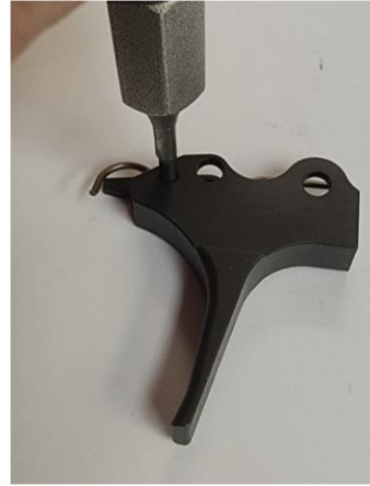
Seat Trigger Spring Pin using 5/64" Roll Pin Punch.
