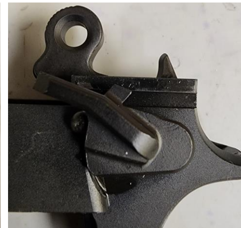
Thumb Safety is “keyed” to the Ejector. Rotating the Ejector down 90 degrees allows the “key” on the Thumb Safety to align with the rectangular hole in the Ejector. The Thumb Safety can now be removed from the frame by pulling Thumb Safety to the left. Be sure not to lose the spring and detent.
