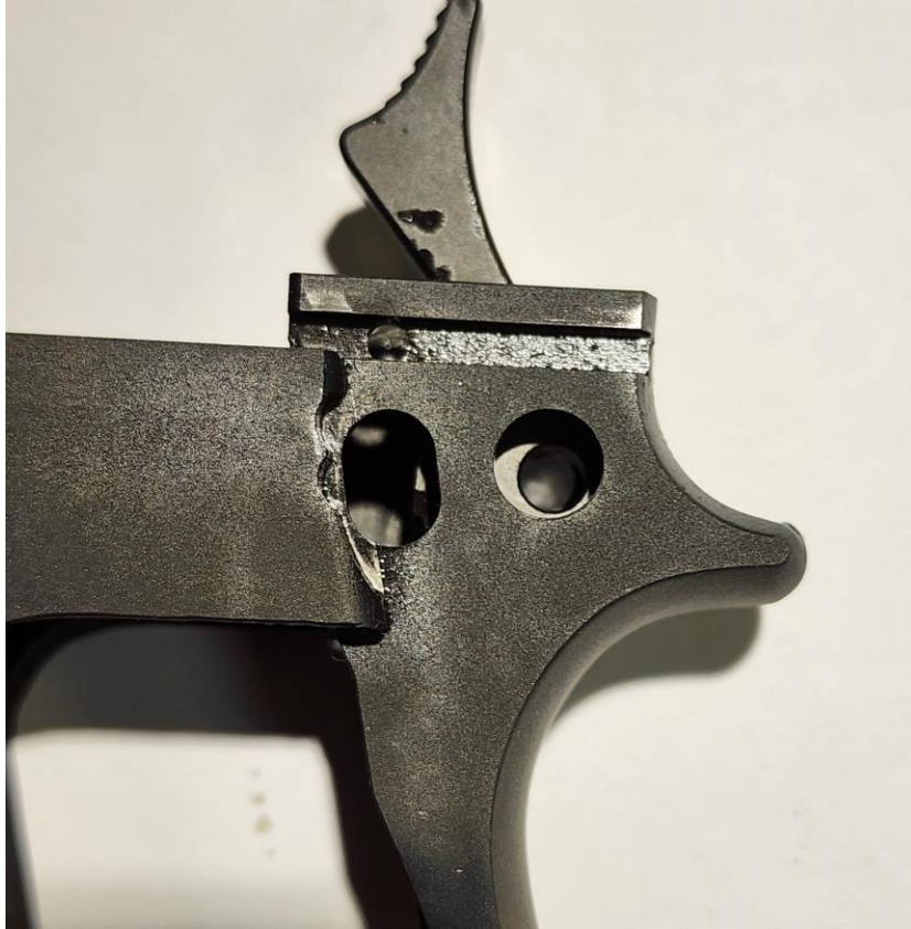
Align Hammer and Frame holes as shown.
