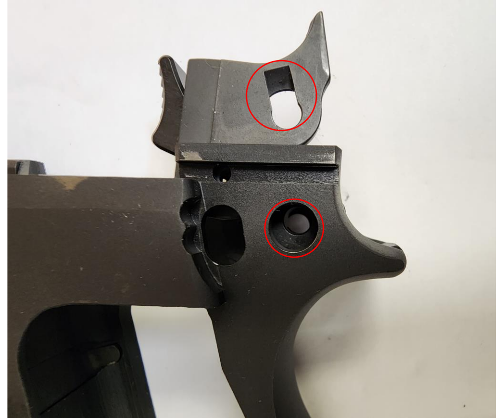
Insert ejector and align keyed hole with Hammer and Frame holes.
