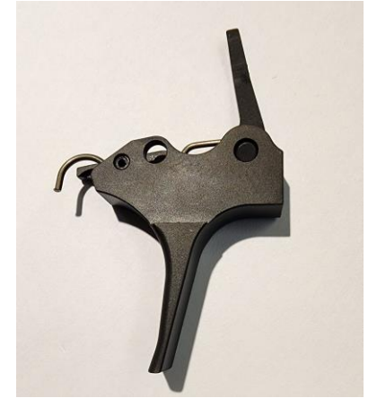
Tail of Trigger Spring will rest in groove in Trigger Lever
