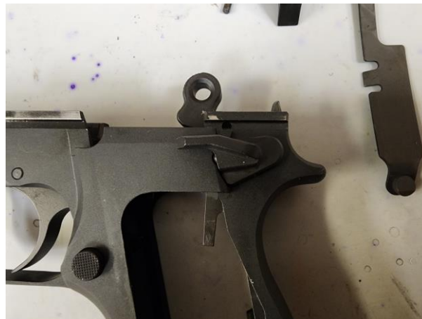
Thumb Safety is “keyed” to the Ejector. Rotating the Ejector down 90 degrees allows the “key” on the Thumb Safety to align with the rectangular hole in the Ejector. The Thumb Safety can now be removed from the frame by pulling Thumb Safety to the left. Be sure not to lose the spring and detent.
