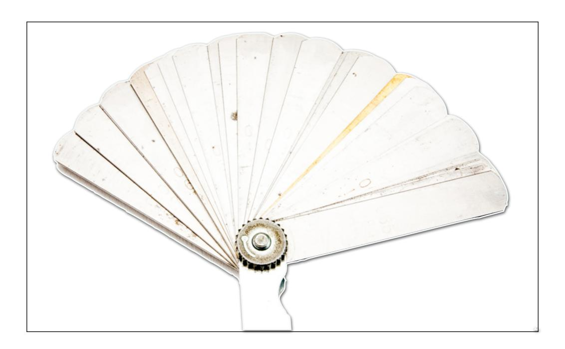
**Step 1:** For proper installation you'll want to use feeler gauges. Arrange the feeler gauges to measure approx. 0.067", give or take 0.001". This measurement may vary based on which trigger you are installing.
