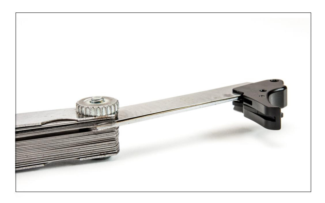
**Step 2:** After ensuring you have a smooth jawed vise, or smooth jaws installed, use your feeler gauges to fill the trigger bar slot between the trigger body's internal structure and the dust shield.
