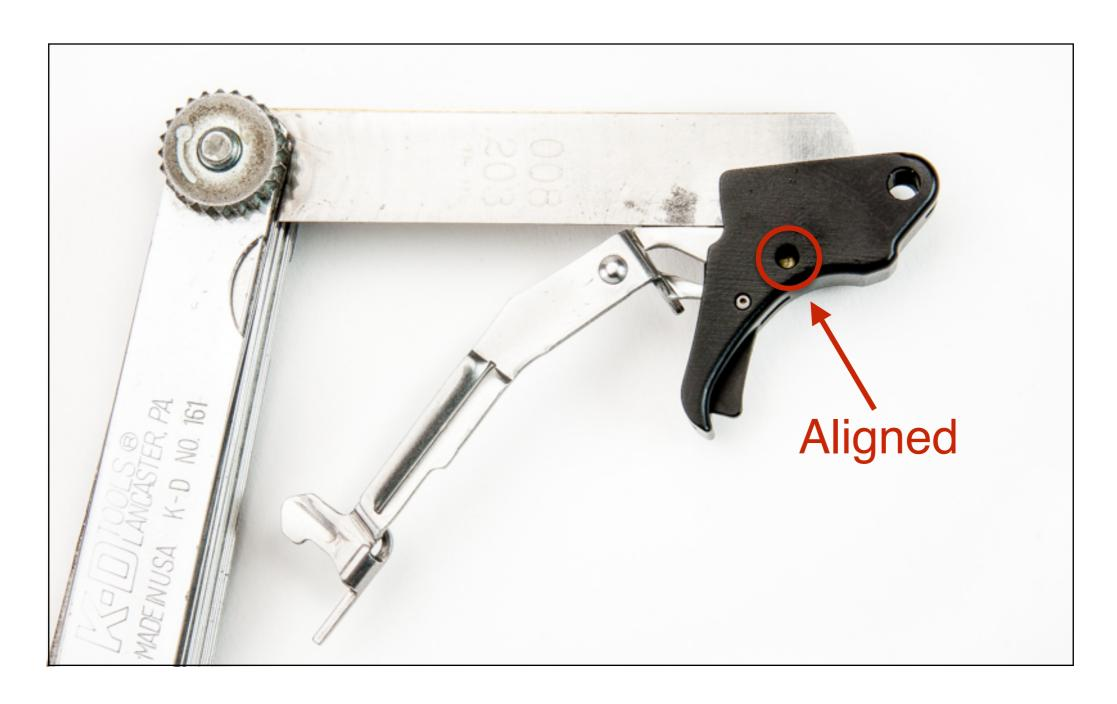
**Step 4:** With the feeler gauges snugly in place, insert the trigger bar into the trigger bar slot and align the trigger bar's pivot hole with the trigger pivot pin hole.
