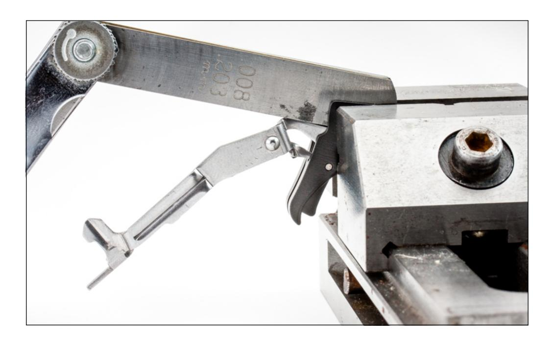
**Step 7:** While holding the feeler gauges and the trigger bar, place the trigger in the vise and squeeze until snug.
