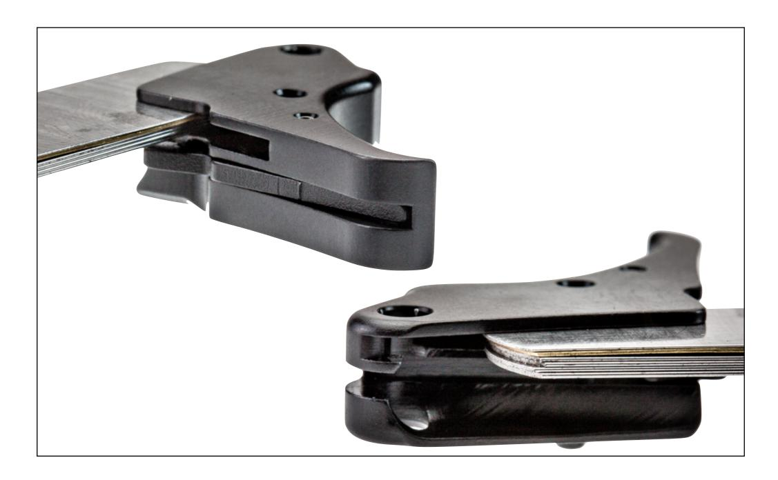
**Step 3:** The feeler gauges should have a snug fit, with little give and without damaging or flaring the trigger body. This is where the trigger bar will be placed.
