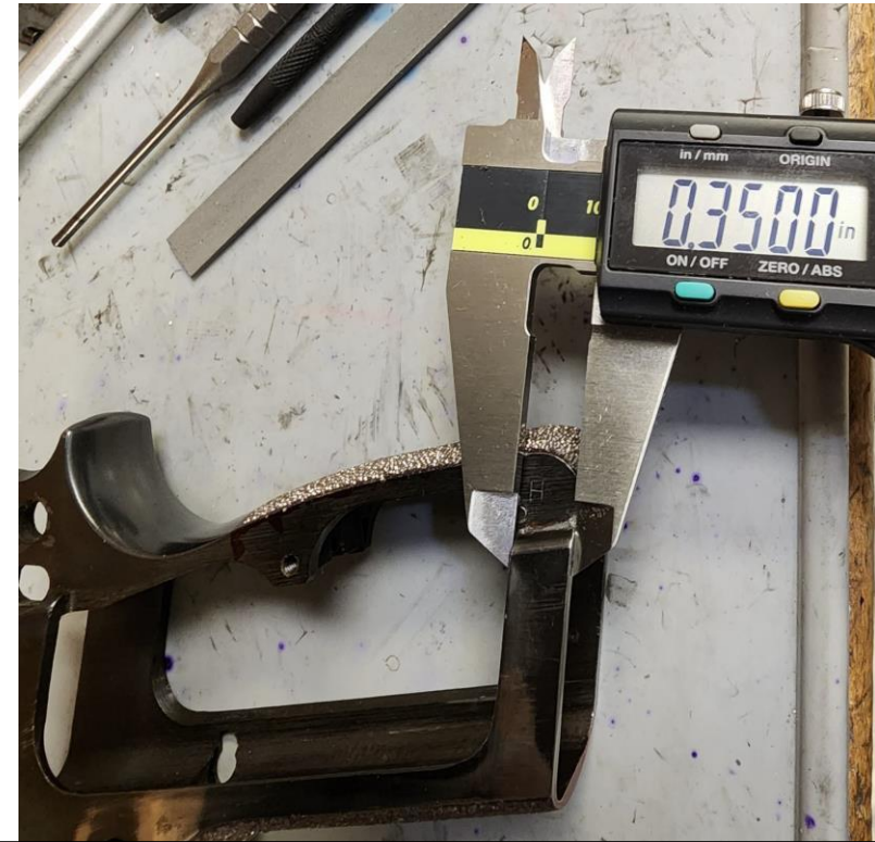
Frame lip filed to correct dimension – both sides of frame 0.350
