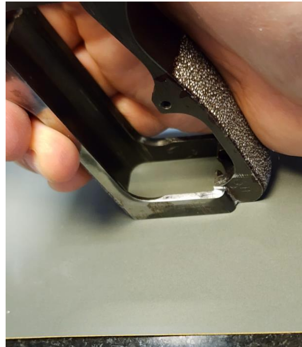
True up bottom of frame
