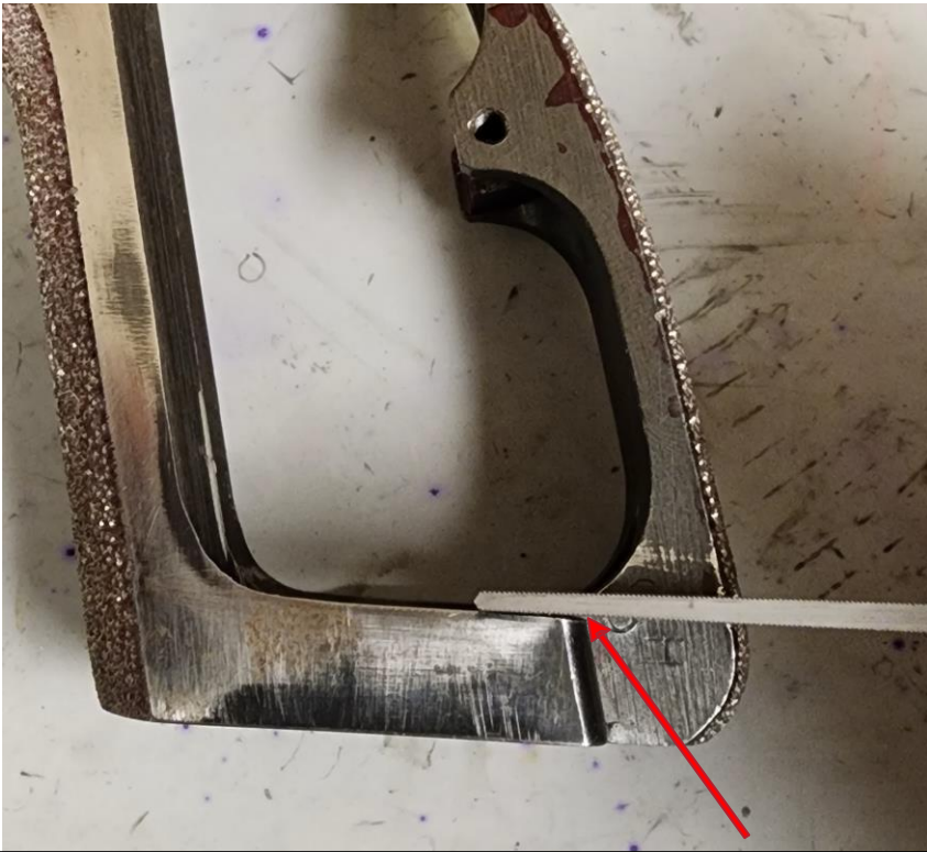
File raised lip on frame to correct dimension
