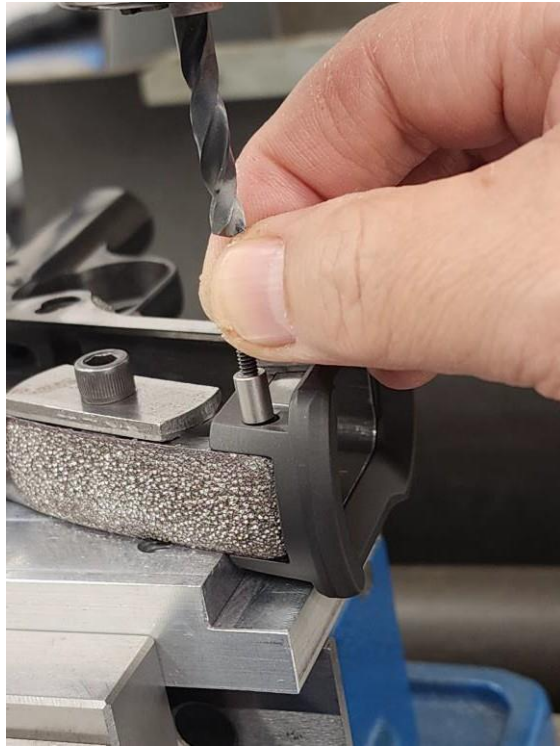
Raise quill or drop milling table. Use 4-40 Screw to insert Anchor Bushing into drilled hole
